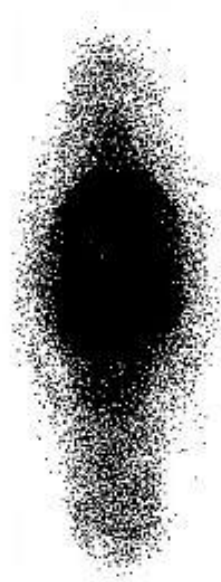
NOT ENOUGH AIR FLOW
