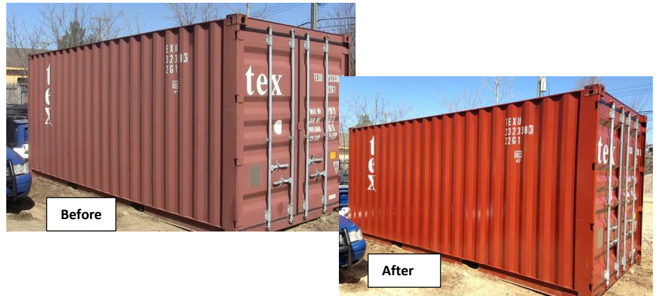
Before and After Application of Protective Coating on a Container Using NCIM
